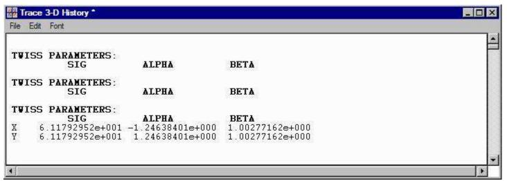
In addition to the X and Y Phase Advances (SIG), TRACE 3-D also computes the X and Y Twiss Parameters for the matched beam (ALPHA, BETA).
