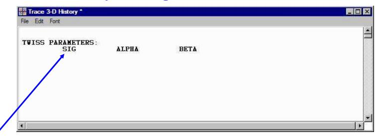
TRACE 3-D first attempts to calculate the phases advances, called "SIG" in this text output. TRACE 3-D "SIG" is in degrees.
