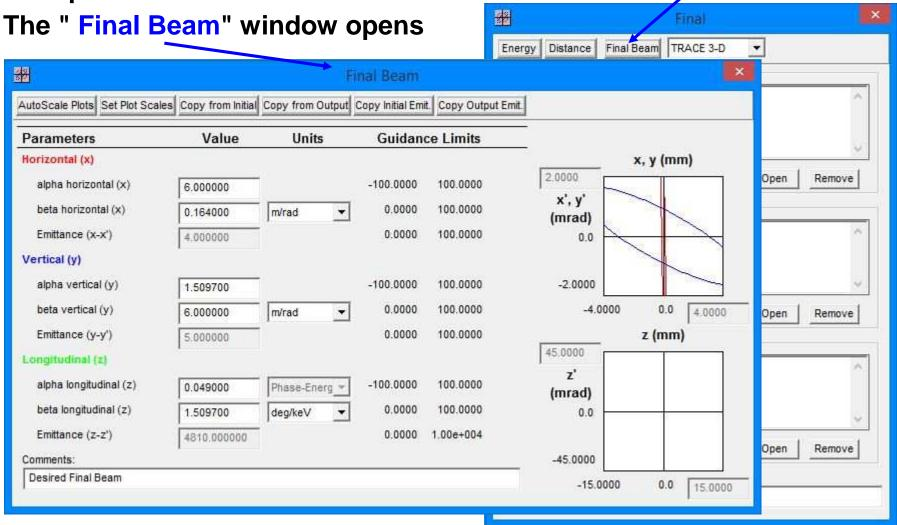
At This Point, One Could Enter the Desired Matched Beam Parameters: i.e. Open the Initial Beam, Copy  $\alpha$  and  $\beta$  Values into Final Beam window
